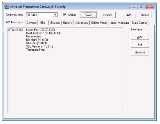
In the Devices tab you will see the IP address of the terminal, Parameters shows the ip address and port which should be 12000.
